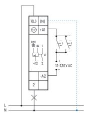
**or** control voltage 230 V with glow lamp current up to 5 mA
